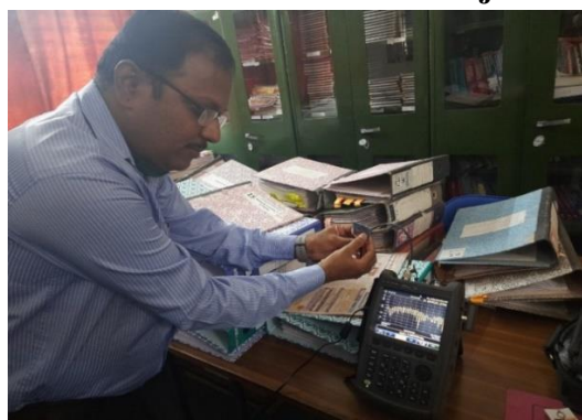
Figure 7: Measurement of compact wearable patch antenna fabricated on jeans material carried out using Agilent Fieldfox N9916A Dual Port Vector Network Analyzer in an open environment.
