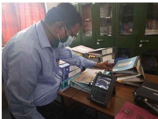
Figure 5: Measurement of compact wearable patch antenna fabricated on cotton material carried out using Agilent Fieldfox N9916A Dual Port Vector Network Analyzer in an open environment at Department of Electronics and Telecommunication, Amrutvahini College of Engineering, Sangamner.
